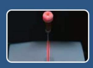
Laser cross hair to align to center of needle hub
