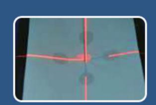
All 4 needle shadows to be aligned to the laser cross hair
